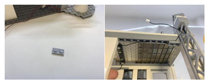
Connect the cables of the lights to the 6 -port Expansion Boards, secure the board in place with adhesive squares
