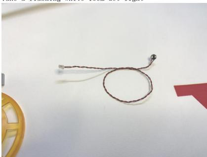
With lighting part facing down, connect the light to the hole at the center of the disc. Note: do not thread it through.
