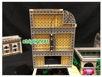
Connect one of the 15cm cables from striplight#1 to the last available port on the expansion board underneath and thread the other connecting cable up the open space which leads to the second level.
