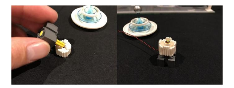
Note: Because of the dot light cable. the 2 sections (white round brick and dark grey brick) will not fully connect and there should be a slight 1-2 mm gap between the two.
