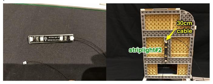
Connect the connecting cable from the level below into the other port on striplight#2 and thread the 30cm cable connected to the other port up the open space which leads to the 3rd level.
