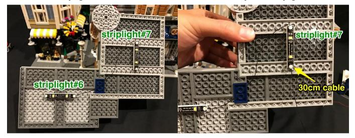
To prevent the cable from hanging down and being seen from the outside looking in, connect LEGO pieces over the top.
