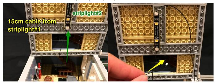
Reconnect the third level on top and then pull the connecting cable up from underneath ensuring it is threaded behind the staircase.
