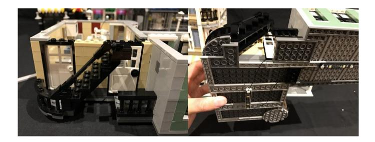
30.) Connect the other end of the 15cm cable from striplight#4 to one of the available ports on the expansion board in the flower shop then reconnect the entire second level back on top.
