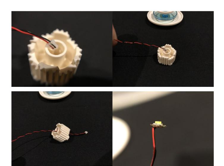
Pull the cable all the way through from the other side so that the LED component is right up against the inside of the white round LEGO piece then reconnect the dark grey brick with yellow technic pin through the top of the white round piece. Your base of the fountain section with blue dot light installed should look similar to the below example.
