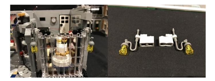
21.) Disconnect the trans yellow piece from each of the lamp sections. Take a Dot Light with 15cm cable and thread the connector side through the larger hole of the trans yellow piece. Thread it all the way through but before the LED component reaches the LEGO piece, bend the component part 90 degrees upward so that the LED component is facing up toward the inside, then pull the cable all the way through.
