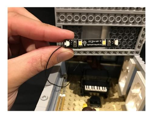
Take the roof of this section of the assembly square and place it on top. Install striplight#3 to the following position and secure the connecting cable in place by laying it underneath one of the grey tiles on top.
