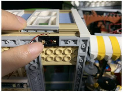
Connect the strip light to the following place, secure the cable by connecting the plate over
