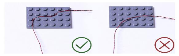
Insert the connectors to the ports.
