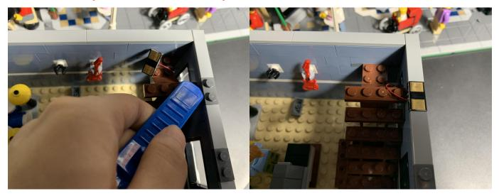
Reconnect the second floor, turn the power on to see if the lighting are working OK
