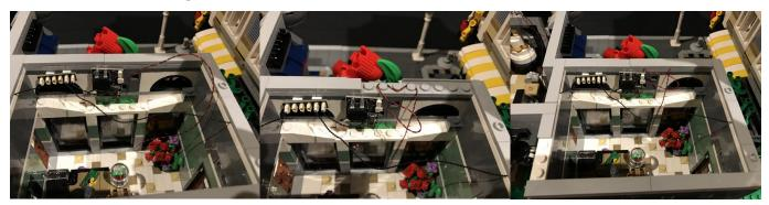
26.) Take a Warm White Dot Light with 30cm cable and connect it to the top port of the multi effects board. Set the other end of this cable aside for now as we will later use this for the flame of the bbq on the top floor.
