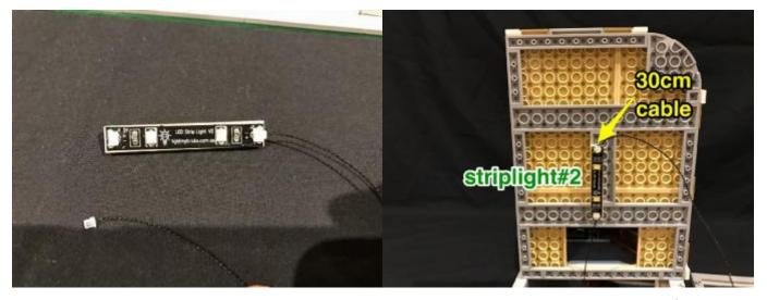
Connect the cable from the second floor to the other port on the striplight#2(connect the
