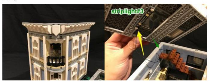
Reconnect the roof. This completes installing the lights for the left part of the square. Connect the cable of the battery pack to the port on striplight#3, turn the power on to test the current. (for the RGB strip light, after turning the power on, remove the battery separator from the remote, turn the strip light on by turning on the switch. Note: remote should be close to the RGB board as much as possible)
