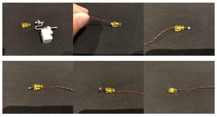
Reconnect the trans yellow piece with dot light installed back to the lamp section ensuring the cable is facing toward the back.
