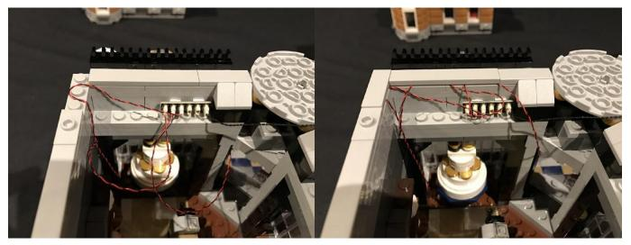
23.) Take the Multi Effects Board and then connect this to another 6-port Expansion board using a 5cm connecting cable. Connect the cable into the port on side of the effects board which only has one port.
