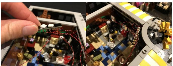
15.) Take a 30cm connecting cable and connect it to one of the spare ports on the expansion board. Take the other end of the cable and thread it through the green vine pieces and then through to the inside of the flower shop.
