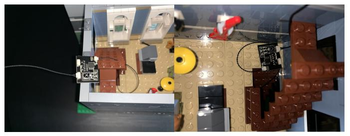
18.) take a white LED (or RGB) strip light, which we'll identify as striplight#2, connect a 30cm connecting cable (or a 15cm RGB connecting cable) to its port. Connect the third floor back, turn it over to its side, connect the striplight#2 to the following place
