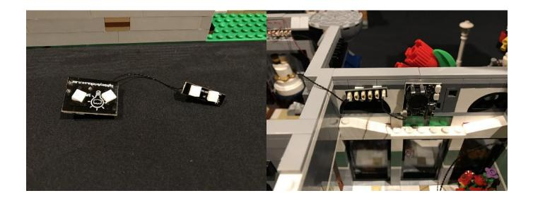
Lay the 15cm connecting cable in between studs underneath the grey tile.
