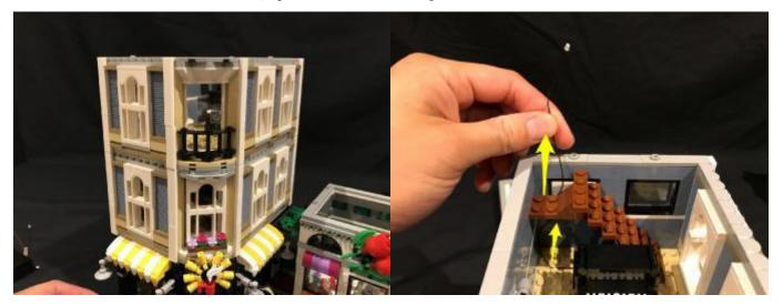
19.) take another strip light (or another RGB strip light), which is identified as striplight#3, connect the cable we pulled up from the lower floor to its left port
