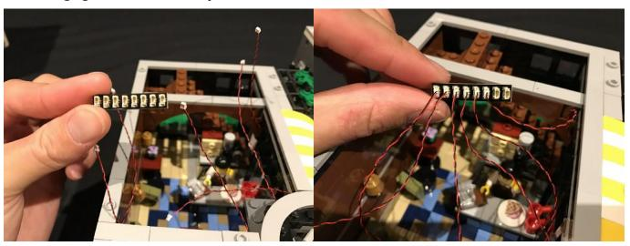
13.) This is a good time to test our current light circuit. To do so, insert 3x AA batteries to the battery pack and then connect the battery pack cable into a spare port of the expansion board. Turn on the battery pack and verify that all the lights connected to the cafe are currently lit.
