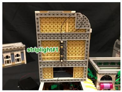
Connect one of the 15cm cables from striplight#1 to the last available port on the expansion board underneath and thread the other connecting cable up the open space which leads to the second level.
