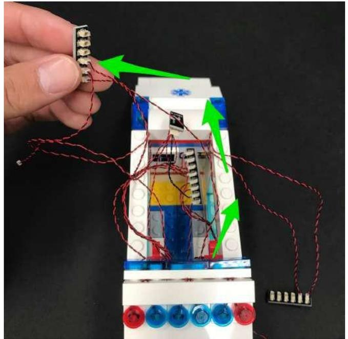
Take the dot light on the left side and connect it to the 6-port expansion board on the right side.
