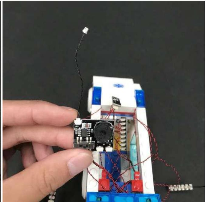
Connect the other end of the 5cm connecting cable from the effects board to the remaining port on the 6-port expansion board (where the head and tail lights are connected to)
