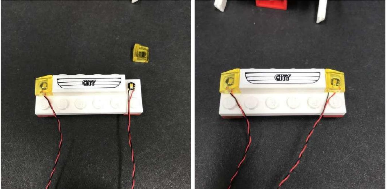
3.) Reconnect pieces we removed earlier ensuring the cables underneath are laid in between studs.
