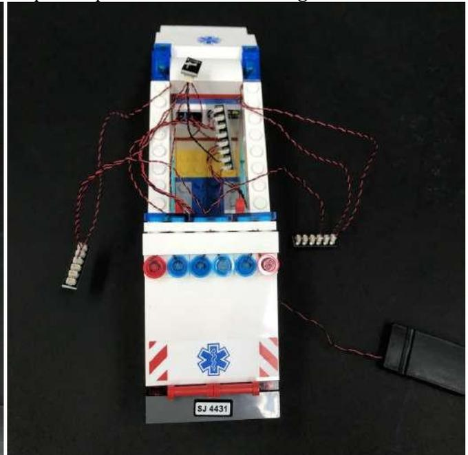
35.) Take the 2x 5cm Connecting Cables and connect each one to each of the 6-port expansion boards on each side.
