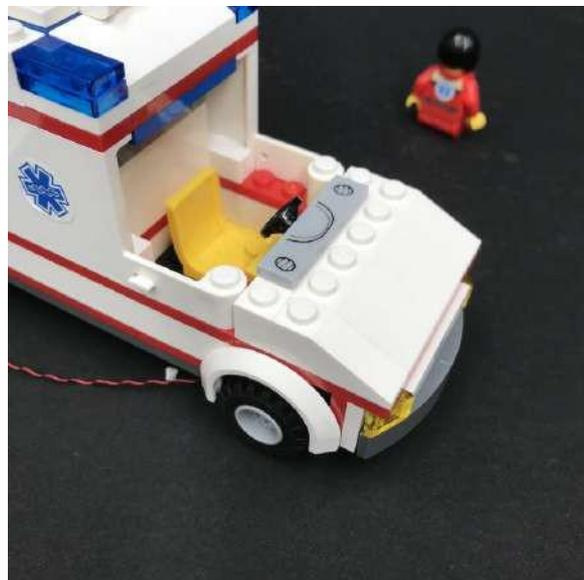
4.) Thread each cable up the space behind the front wheels. Pull the cables up from the top and then tuck the cable in over the wheel.
