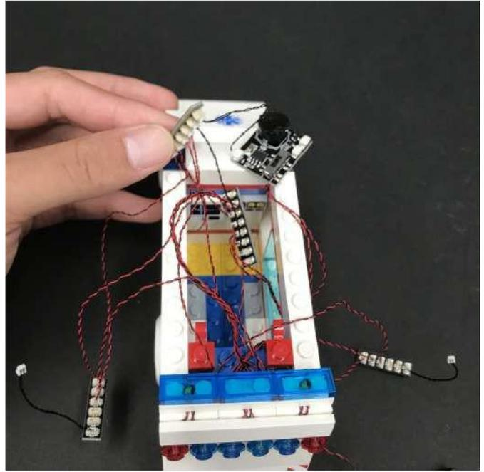
37.) Take the spare ends of the 2x 5cm Connecting Cables from the expansion boards (where the roof lights are connected to) and connect each one to the output ports of the multi effects board (side with 2 ports)
