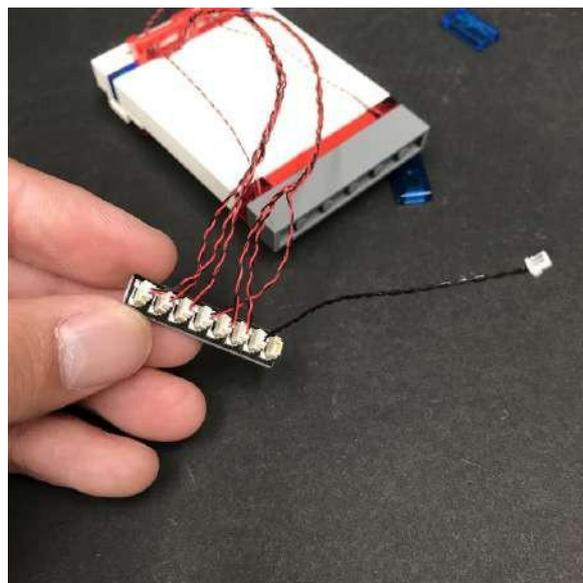
26.) Take this time to test the flashing lights we have just installed. To do this take the Flat Battery Pack and insert 2x CR2032 batteries to it. Connect the battery pack to the spare port on the expansion board and then turn it on to ensure flashing lights are working OK.
