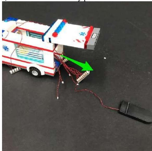
32.) Locate the 6-port expansion board with the headlights connected to it and then bring the tail lights back in from the back of the ambulance and connect them to it.
