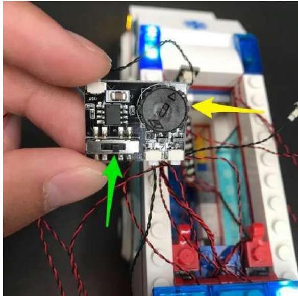
39.) Once you have configured the effect to your desired speed, neatly tuck all the components inside the back of the ambulance.
