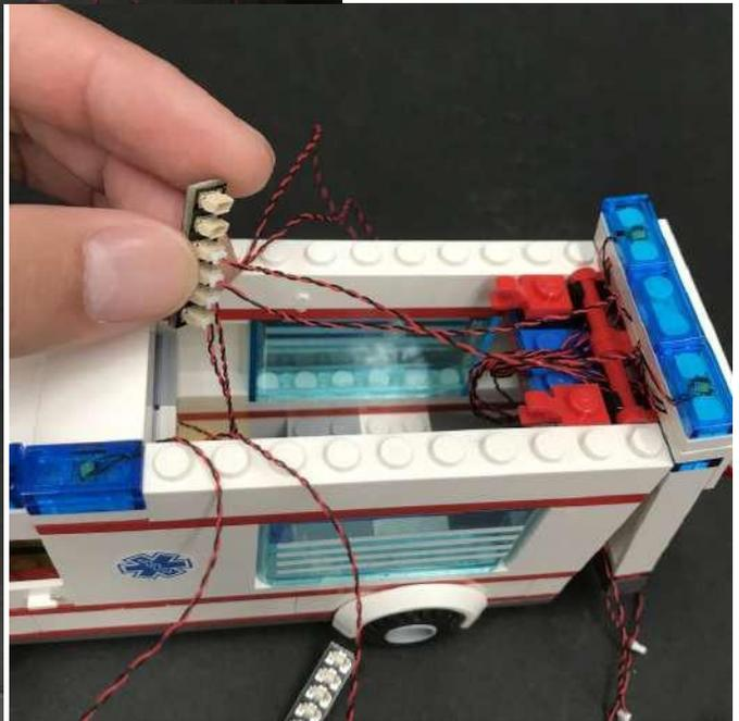
Locate the other end of the 5cm connecting cable from the 8-port expansion board and bring this back in and connect it to the 6-port expansion board inside (where the head and tail lights are connected to)
