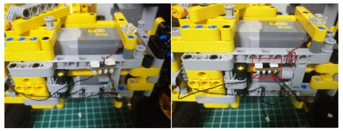
Take a USB cable, a Remote Control Switch Board, connect the USB cable to the port underneath the  $5V\mathcal{-IN}$  as per below.
