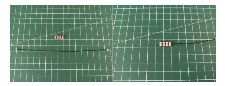
Connect the following cable to the expansion board.
