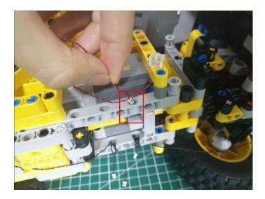
Wind the cable around the following piece several times.
