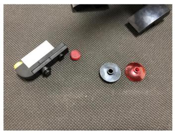
Take a 30cm red dot light, thread the light through the black round plate with hoe, pull the cable out till the light is placed against the hole.
