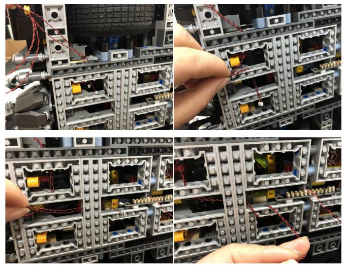
Connect the cable to the 12-port expansion board.
