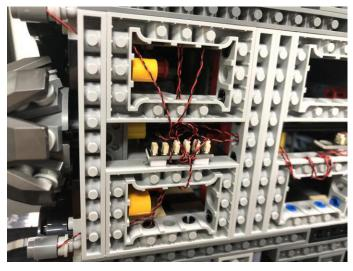
Take two 5cm connecting cable, a Flicker Effects Board, connect the two cables to the input and output ports of the Flicker Effects Board.
