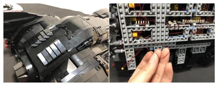
Thread the cable of the battery pack through the hole, and connect it to the 12-port expansion board.
