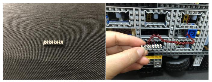
Tuck excess cables, and stick the expansion board to the following place with the adhesive squares.
