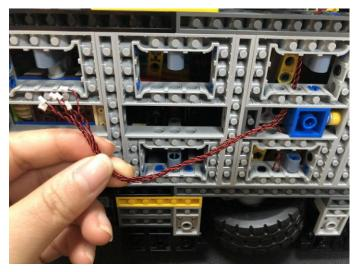
Take an 8-port expansion board, connect the 6 cables of the lights to it.
