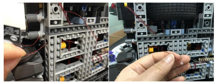
Take a 6-port expansion board, connect the 2 cables of the lights to it.
