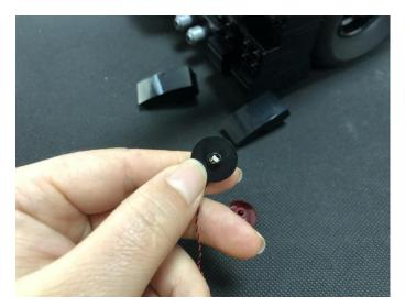
Secure the light with the trans red plate.
