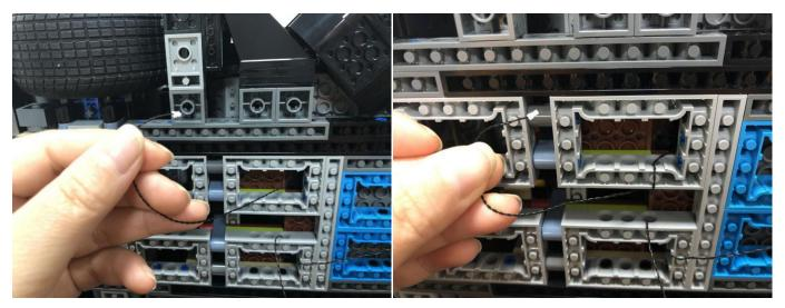
Take a 12-port expansion board, connect the cables of the strip lights and the connecting cable from the expansion board with headlights cables to it.
