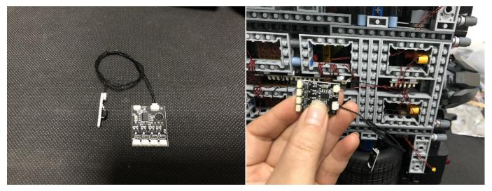
Take a 5cm connecting cable, connect it to one of the output port on the Remote Control Switch Board.
