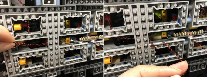
Connect the cable to the 12-port expansion board.
