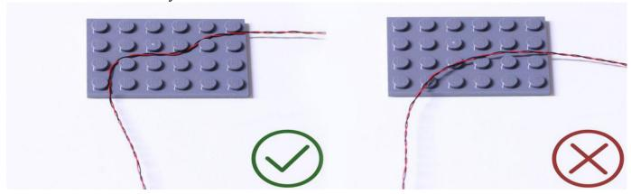
Insert the connectors to the ports.
