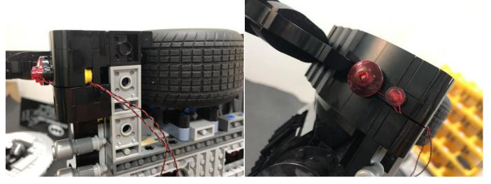
Thread the cable through the holes underneath the car(thread it randomly), and pull it to the 12-port expansion board.
