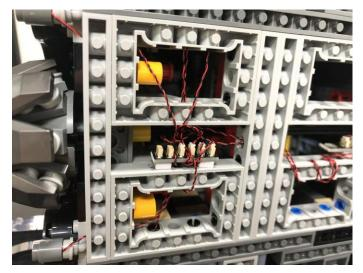
Take two 5cm connecting cable, a Flicker Effects Board, connect the two cables to the input and output ports of the Flicker Effects Board.
