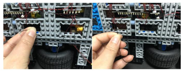
Tuck excess cables, connect it to the 12-port expansion board.
