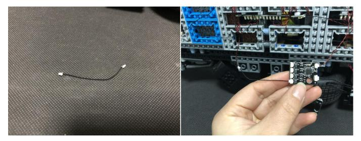
Connect the 5cm connecting cable to the 12-port expansion board.
