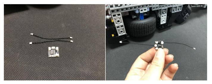
Connect the other end of the cable from the output port to the 6-port expansion board, connect the one from the input port to the 12-port expansion board.
