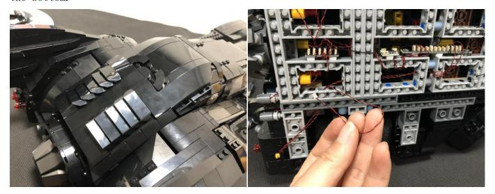
Take the Remote Control Switch Board, connect the connecting cable to the Remote Control Switch Board.
